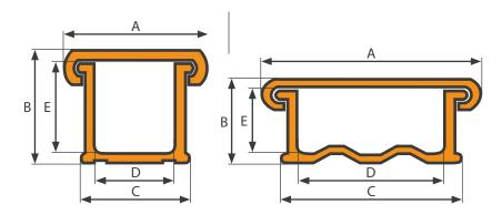
Castioni GRP cable ducts made of glass fibre reinforced polymer are manufactured using the pultrusion process.Some pultruded GRP cable ducts are available from stock and are used in a wide variety of cable management applications.GRP cable ducts are used in highly corrosive environments such as in road tunnels or in subway shafts, train tunnels, offshore installations, alongside railway tracks, in industrial sectors and much more.
